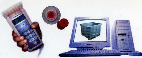
RF (radio frequency) ID containers have embedded microchips, which are either programmable or have fixed serial numbers. Data in ID containers can be read into computers using hand scanners or scanners installed in forklifts or conveyor belts. A wide selection of software is available for managing the entire production process using ID containers at all stages from the slaughterhouses to value added processing. ID containers offer enhanced security and automation of the production process.
