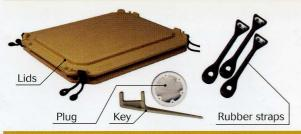
All Borgarplast containers can be fitted with lids, which are insulated with Polyurethane (PUR). Lids are fastened to the containers with strong rubber straps, which are resistant to ultraviolet light (UV), but are not considered fully watertight. Completely filled containers with lids are stackable on top of each other.
